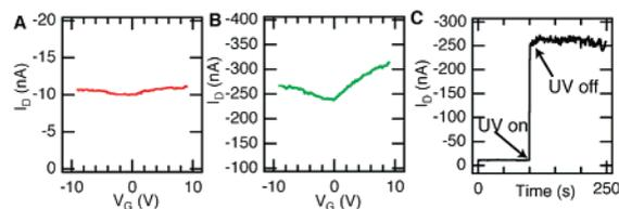
**Figure 2.** (A) Individual SWNT device connected with open-**1**. (B) Device from (A) after UV irradiation to form closed-**1**. (C) Drain current as a function of time.  $V_{SD} = -50$  mV.  $V_G = -9$  V.
