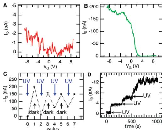
**Figure 3.** (A) Individual semiconducting SWNT device connected with open-2. (B) Device from (A) after UV irradiation to form closed-2. (C) Drain current as a function of the switching cycle for the device is irradiated with UV light and then left in the dark for 12 h. For (A)–(C) the  $V_{SD} = -50$  mV and  $V_G = -9$  V. (D) Steps in the conductance for a device reconnected with 2 when the UV light is pulsed.  $V_{SD} = -50$  mV and  $V_G = -1$  V.
