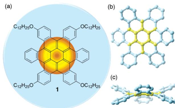
**Figure 1.** (a) Structure of contorted tetra(dodecyloxy)hexabenzocoronene (HBC) **1**. The hexaradialene core is highlighted in orange and the insulating cladding in blue. Crystal structure (from reference 1) showing the (b) face-on view and (c) side-on view of the compound with the hydrogens and sidechains removed to clarify the view. The low-energy hexaradialene core is shown in yellow and is surrounded by the alkoxyphenyl cladding in blue.
