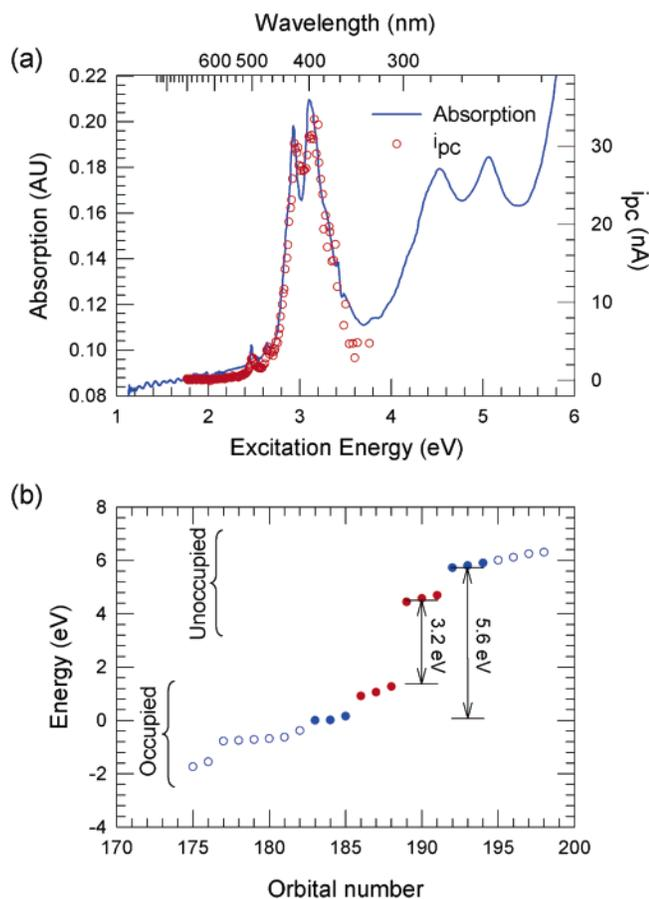
**Figure 2.** (a) Optical absorption spectrum (solid line) and photocurrent spectral response (circles) of tetra(dodecyloxy)-hexabenzocoronene thin films. The photoconductivity is shown for an electric field of  $2.87 \times 10^5$  V/cm. (b) Molecular orbital energies of tetra(methoxy)hexabenzocoronene calculated by DFT.
