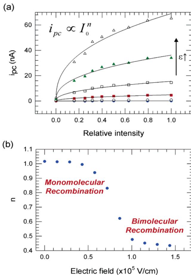
**Figure 4.** (a) Intensity dependence of the photocurrent for the HBC thin films at applied electric fields of (●) 0 V/cm, (○)  $5.74 \times 10^4$  V/cm, (■)  $1.15 \times 10^5$  V/cm, (□)  $1.72 \times 10^5$  V/cm, (▲)  $2.3 \times 10^5$  V/cm, and (△)  $2.87 \times 10^5$  V/cm. The excitation energy was 3.1 eV (400 nm). The solid lines are nonlinear least-squared fits to  $y \propto x^n$ . (b) Power values,  $n$ , of the function  $i_{pc} \propto I_0^n$  vs electric field.
