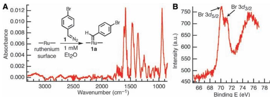
**Fig. 1.** To form the monolayer **1a**, a fresh ruthenium surface reacted with 4-bromophenyldiazomethane (**1**). (A) Surface polarized IR spectrum. (Inset) Reaction of a ruthenium surface with 4-bromophenyldiazomethane to give a derivatized surface. (B) XPS showing the presence of bromine atoms. a.u., arbitrary units.
