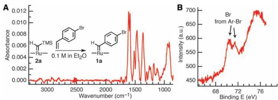
**Fig. 2.** Conversion of **2a** into **1a** with the use of a 1 mM solution of 4-bromostyrene in ether. (A) IR spectrum. (Inset) Reaction of derivatized surface **2a** with 4-bromostyrene to give derivatized surface **1a**. (B) XPS from the bromine after reaction. a.u., arbitrary units.
