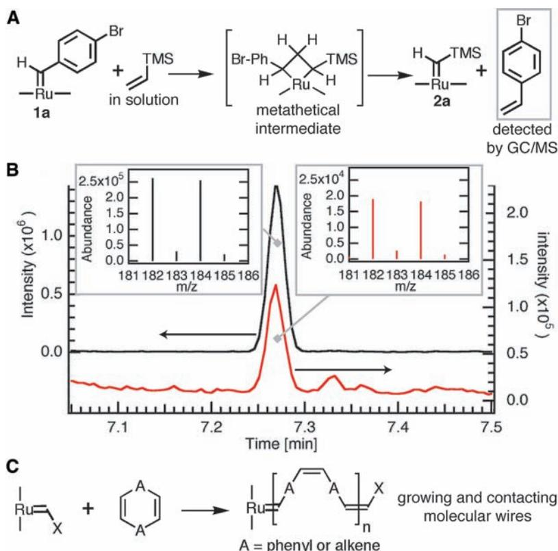
**Fig. 3.** (A) Reaction of **1a** with vinyl-trimethylsilane through a surface metathesis reaction to yield **2a** and 4-bromostyrene. (B) The 4-bromostyrene can be detected by GC/MS. The insets show the characteristic mass and isotope pattern for the 4-bromostyrene standard (left inset) and for the reaction mixture (right inset). m/z, mass-to-charge ratio. (C) Ring opening metathesis polymerization pathway to conjugated molecular wires in electrical contact with a Ru metal particle or surface.
