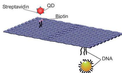
**One on each side:** Gold nanoparticles (AuNPs) and semiconducting quantum dots (QDs) are integrated on a single DNA origami scaffold. Streptavidin-functionalized QDs bind to biotin anchors on one side of the DNA origami, while DNA-coated AuNPs bind through DNA hybridization to single-stranded DNA on the other side of the scaffold. This approach offers a new path toward the organization of complex systems consisting of disparate materials.
