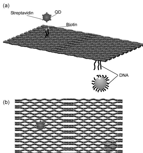
**Figure 1.** Schematic drawings of the assembly of CdSe QDs and AuNPs on opposite sides of a DNA origami scaffold. a) Streptavidin-coated CdSe QDs were attached to biotin-modified DNA anchors on one side, while ssDNA-wrapped 10 nm AuNPs were assembled to the other side through DNA hybridization. b) Schematic showing the binding position of QDs and AuNPs on the DNA origami scaffold.
