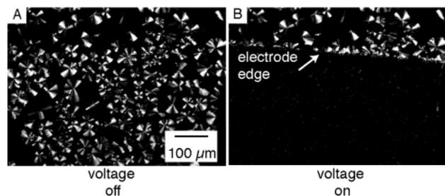
**Figure 5.** **1c** sandwiched between two sheets of ITO coated glass separated by 5  $\mu\text{m}$  at 160  $^{\circ}\text{C}$ : (a) 0  $\text{V}/\mu\text{m}$  field; (b) 20  $\text{V}/\mu\text{m}$  field.
